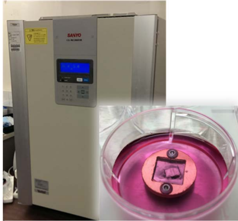
Figure 25. Patterned cpTi foil fixed on a copper cylinder fixture seeded with chondrocytes in a cell culture chamber for cell incubation.
